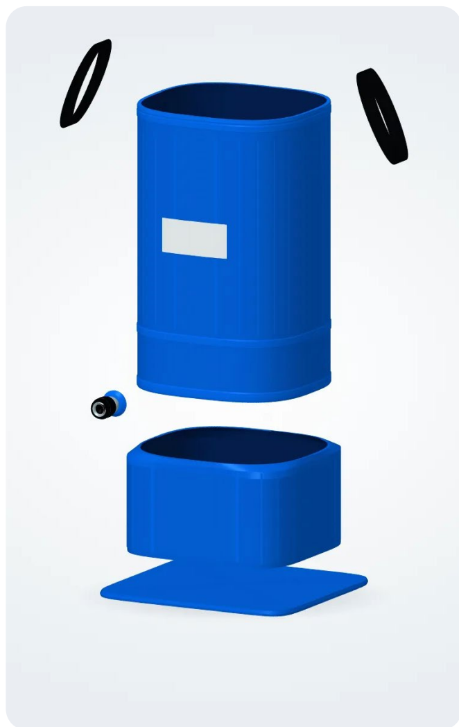
Exploded view: leg, quick coupling, base and sole · 3D study, three-quarter view · 3D study, side view
